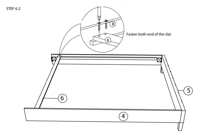
A. Use Screw(K) to fasten one slat(6) at the front side of the SideRail(4) as shown above.
