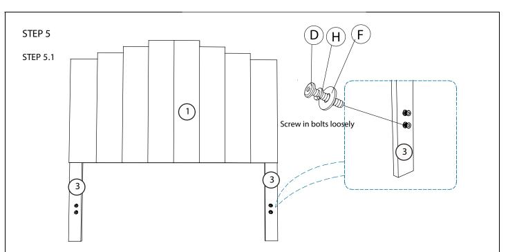
A. Use Allen Key(A) to drive and loosely screw in Bolt(D) fitted with Spring Washer(H) and Flat Washer(F) onto the Headboard Leg(3)
