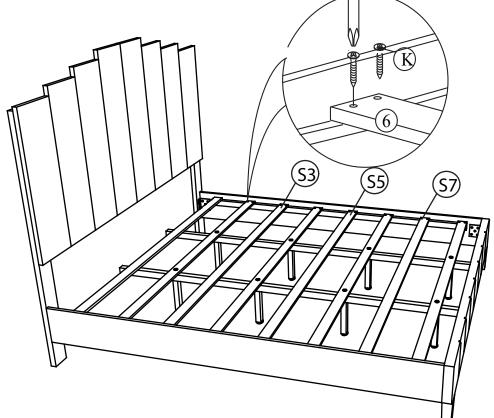
A. Place the rest of the slats(6), denoted as S3, S5 & S7 on the SideRail(4). Use Screw(K) to fasten all the slats(6).
