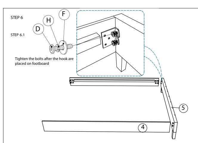
A. Place the hook on Side Rail(4) to the bolt(D) on Footboard(5). Tighten the bolts fully.
