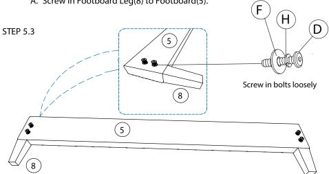
A. Use Allen Key(A) to drive and loosely screw in Bolt(D) fitted with Spring Washer(H) and Flat Washer(F) onto the Footboard(5).
