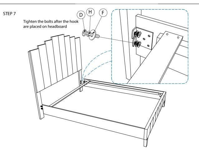
A. Place the hook on SideRail(4) to the bolts(D) on Headboard Leg(3) as shown above.
