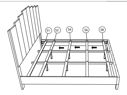
A. Place the assembled slats on the Side Rail(4). Slide in the Center Support Bar(7) underneath the first slat as shown above.
