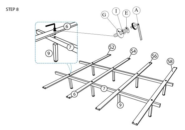
A. With assistance, use Bolt(E) fitted with Spring Washer(I) and Flat Washer(G) to attach 4 pieces of Slats(6) denoted as S2, S4, S6 & S8, to the Center Support Bar(7) and Center Support Leg(9) as shown above.
